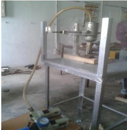
Fig 2 :Set up of Abrasive Jet machine
