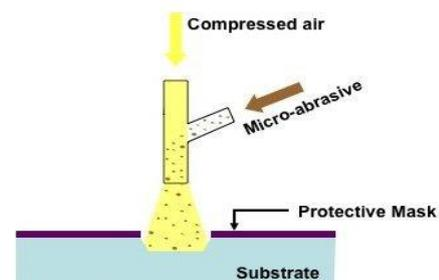
Fig 1 : Process Diagram of Abrasive jet machining
