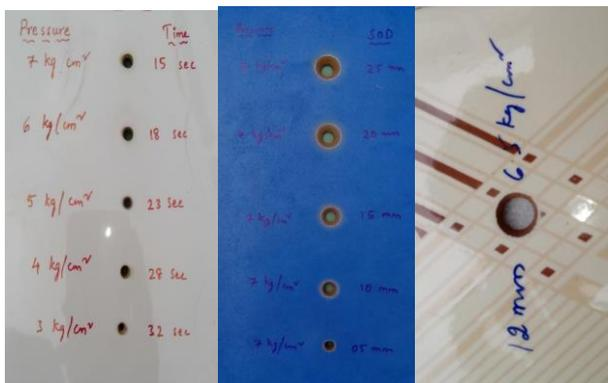
Fig 8: Ceramic tiles drilled at different Pressure, SOD, and AFR
