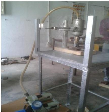
Fig 2 :Set up of Abrasive Jet machine
